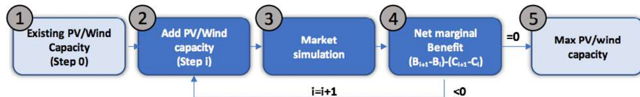
Figure 12.6 - Iterative process to evaluate the maximum PV/wind capacity that can be integrated in the interconnected system
